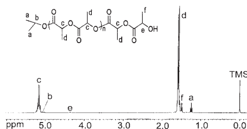
Figure 5 ^1\text{H} -NMR spectrum of poly( rac -LA) (Table I, entry 3; \text{CDCl}_3 , 300 MHz; TMS = tetramethylsilane).
